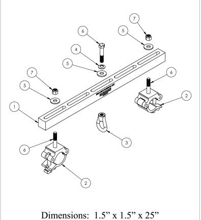
The Mega-Video Wall Hanger works with up to 24-inch truss and has a 500 pound Working Load Limit. Video walls can be center hung or over hung with the Mega-Video Wall Hanger. CNC machined from 6061T-6 aluminum alloy with five 4.4" x .531" slots for attaching Mega-Couplers or suspending video wall sections from the forged steel 1/2" eye nut. The Mega-Video Wall Hanger allows for diagonal attachment to clear truss bracing. Two Mega-Couplers and one Eye Nut with 1/2" steel fasteners are included.
